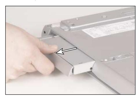
**9** Firmly push the new bay module straight into the bay until the latch clicks into place.
