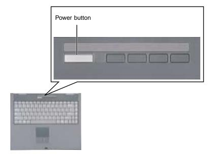
The power button is preset to On/Off mode. However, you can also set it to function in Standby/Resume mode. For instructions on changing the power button mode, see "Changing power settings" on page 151.
