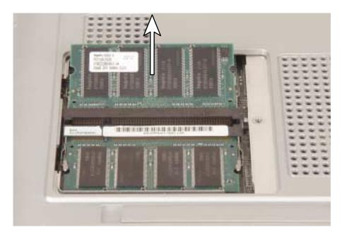
**9** Hold the new or replacement module at a 30-degree angle and press it into the empty memory slot. This module is keyed so that it can only be inserted in one direction. If the module does not fit, make sure that the notch in the module lines up with the tab in the memory bay.
